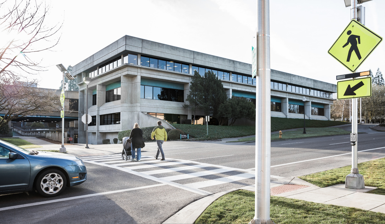
Pedestrian safety projects include pavement marking, signing, and warning devices like this Rapid Rectangular Flashing Beacon
