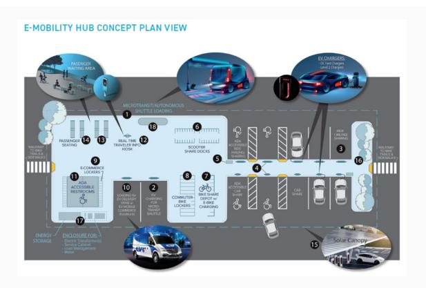
An e-mobility hub incorporates electric vehicle charging and renewable energy into a place of connectivity where different modes of travel are supported.
