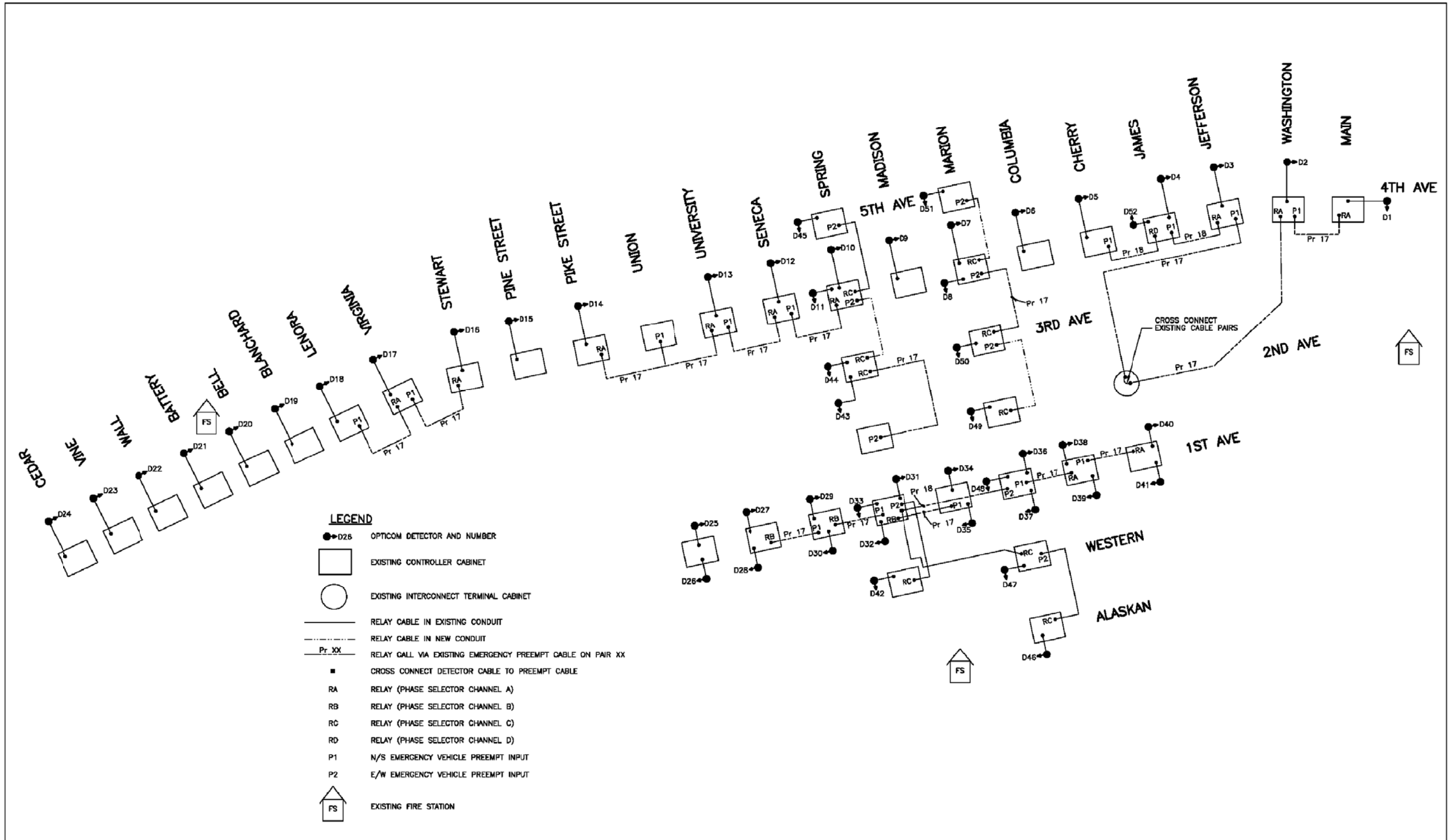
Figure 4: Detector Call Cascading Schematic
